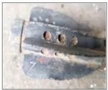
**Figure 6.** 2-inch mortar tailfin as typically found.
