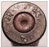
**Figure 3.** 303 cartridge 1943 Headstamp with Lee-Enfield rifle firing pin indent.
